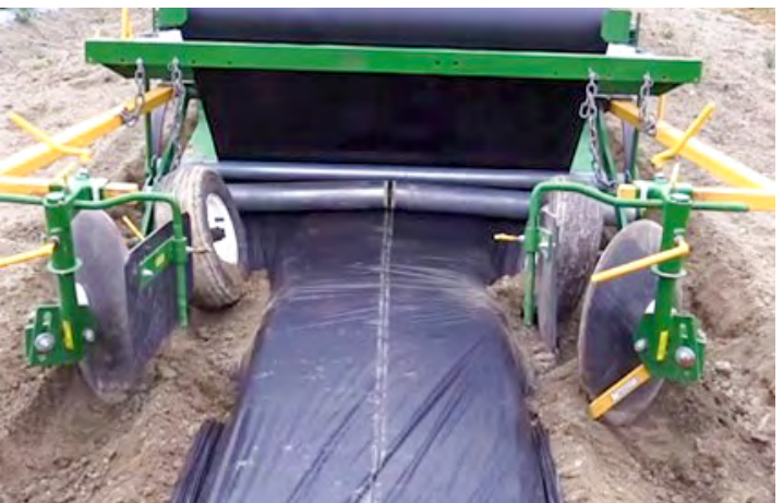
Figure 3. Step on the mulch or use a weight to hold it down before the tractor starts moving forward (above). Mulch layer roller bars should move freely and wheels should barely touch the mulch (above right). The mulch should be loose on the bed to avoid ripping (right); it will tighten after it moistens and dries.
