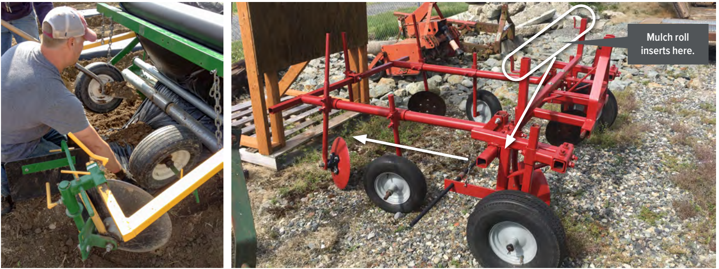
Figure 2. Feeding the mulch through the roller bar in new mulch layer (left). An older mulch layer (mulch roll inserts as shown in white; right).
