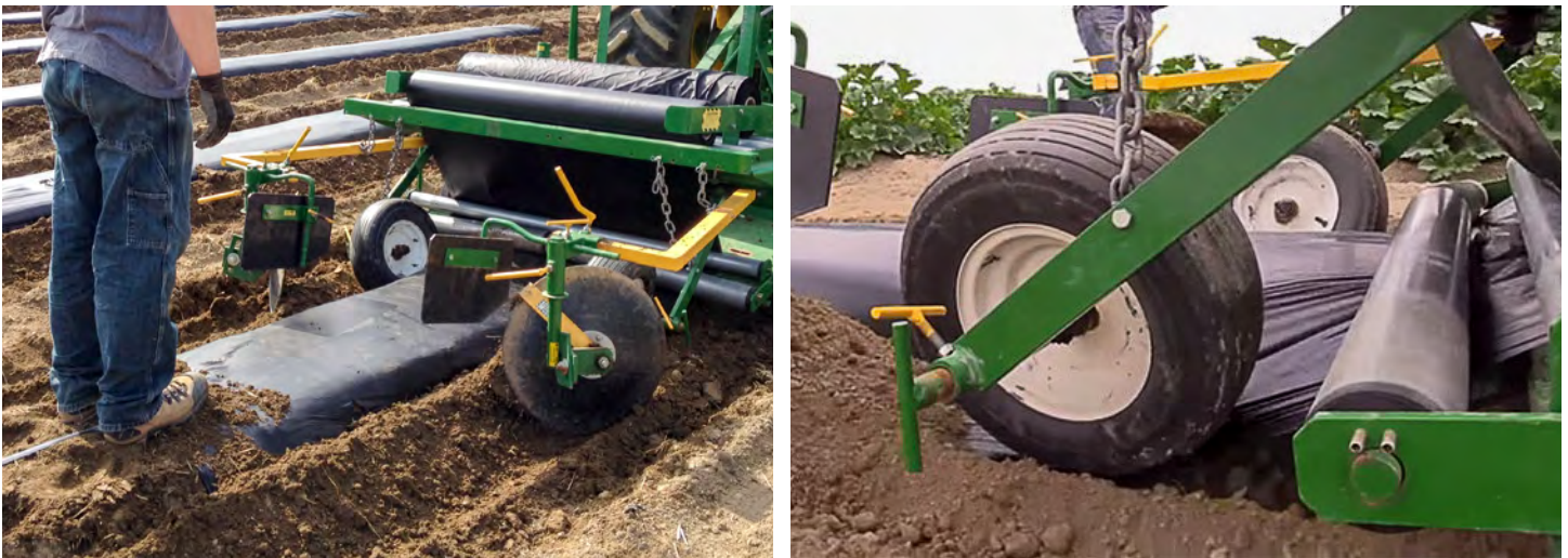
Figure 3. Step on the mulch or use a weight to hold it down before the tractor starts moving forward (above). Mulch layer roller bars should move freely and wheels should barely touch the mulch (above right). The mulch should be loose on the bed to avoid ripping (right); it will tighten after it moistens and dries.
