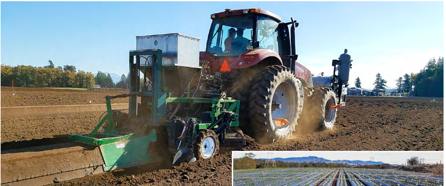
Figure 2. Tractor with bed fumigation attachment that simultaneously makes raised beds and applies fumigant. Mulch will be applied after fumigation (above).
