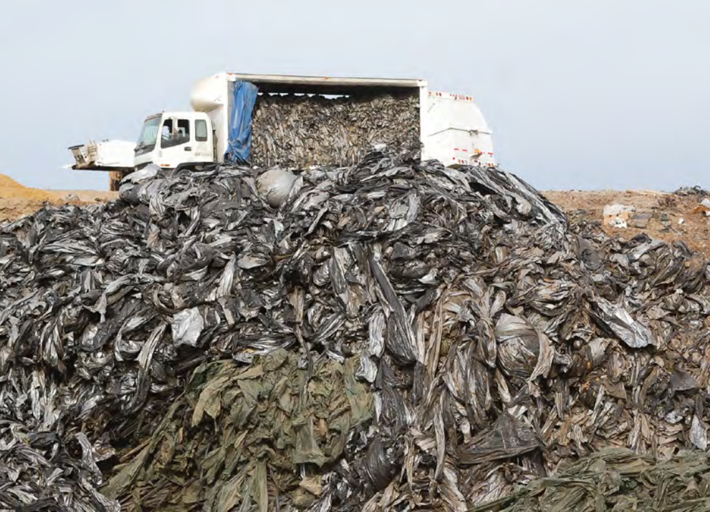
Used agricultural plastics often contain high levels of soil, field organics, and other contaminants. [ReGen Monterey]
