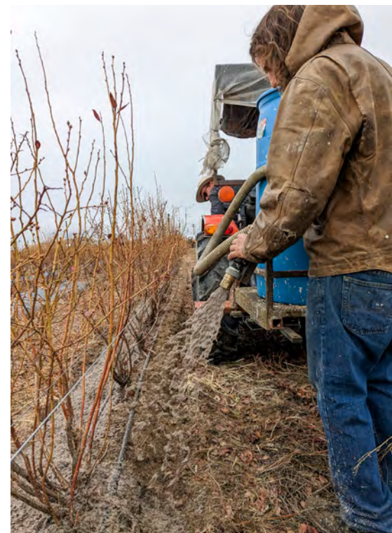
An experimental portable pump system is used to apply small volumes of hydromulch on top of raised beds in a blueberry field.
