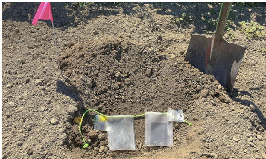
Figure 1. Mesh bags and mulch samples being buried to test the degradation of soil-biodegradable plastic mulch in the field.
