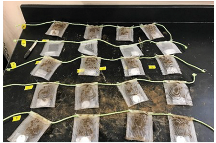
Figure 12. Mesh bags connected with rope and stapled with stainless steel staples.
