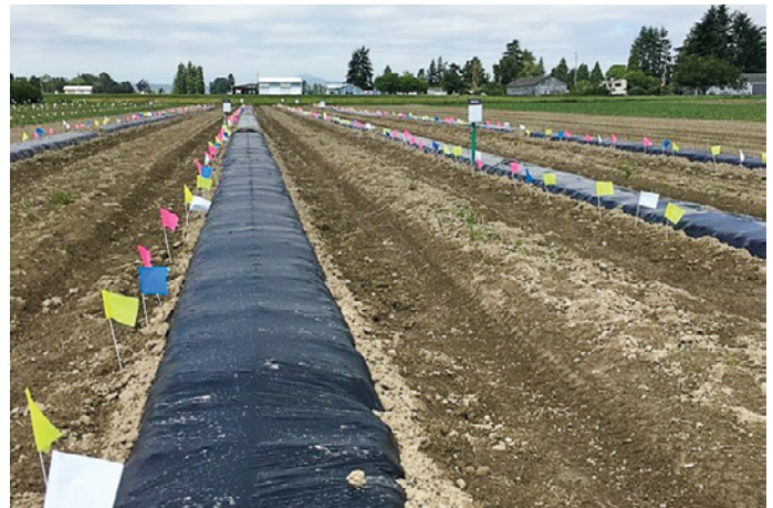
Figure 13. Field experiment with flags marking the burial sites of mesh bags, which are under soil-biodegradable plastic mulch covering a bed.
