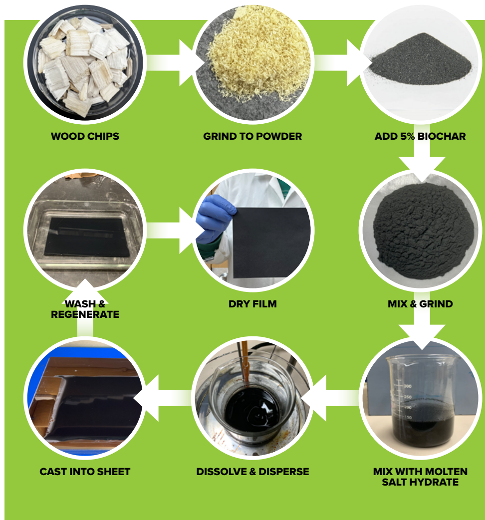
The process of making lignocellulosic film from raw wood chips. Images provided by Haishun Du, PhD Research Associate at University of Wisconsin-Madison.
