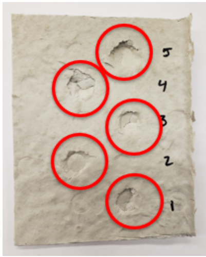
Samples of hydromulches that have been tested for puncture resistance (left) and tensile strength (right).
