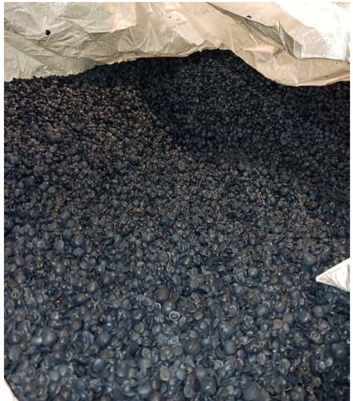
Figure 5. PE mulch following mechanical processing, transformed into plastic pellets.
