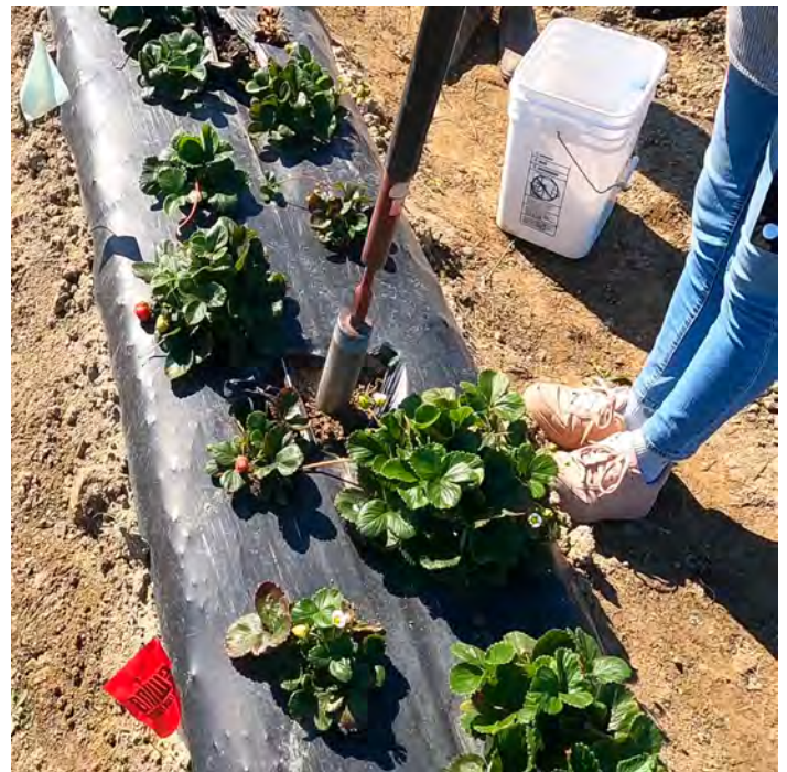
Figure 1. Collecting soil samples for measurement of aggregate stability from the long-term mulch trial in Mount Vernon, WA.
