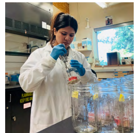
Figure 2. WSU PhD candidate Nayab Gull rewets soil samples to conduct a potentially mineralizable carbon (or soil respiration) assay.
