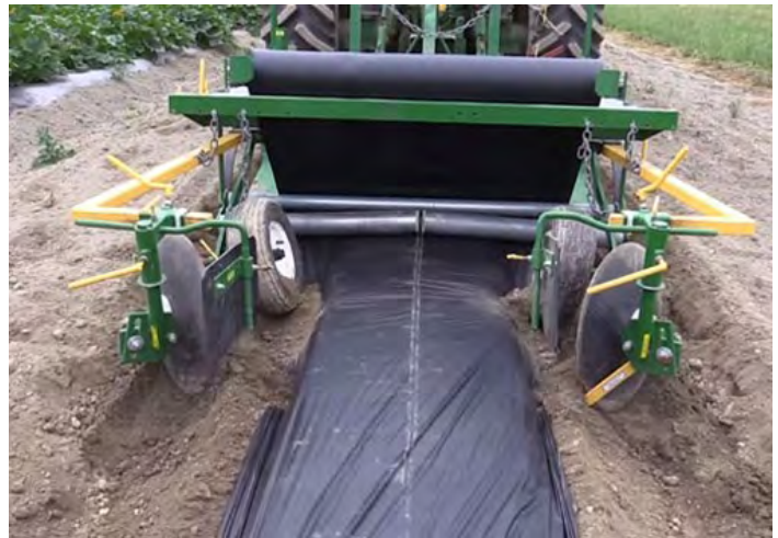
Figure 1. Laying soil-biodegradable mulch (BDM) by machine.
