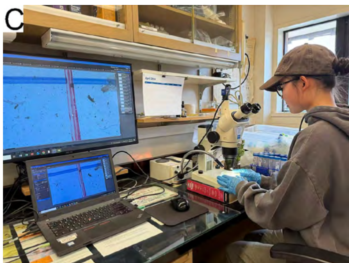
Figure 1. Photographs documenting the microplastic extraction process from soil. (A) Soil and reagent mixtures prepared by Fenton digestion and density separation prior to filtration. (B) Filtration and separation of suspended particles. (C) Stereo microscope used to inspect and select suspected plastic particles for micro-FTIR identification. (D) Image of a filter paper containing extracted microplastics.
