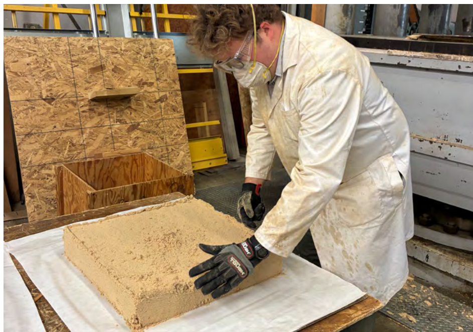
Figure 1. Final surface preparation of a medium density fiberboard (MDF) panel before hot pressing.
