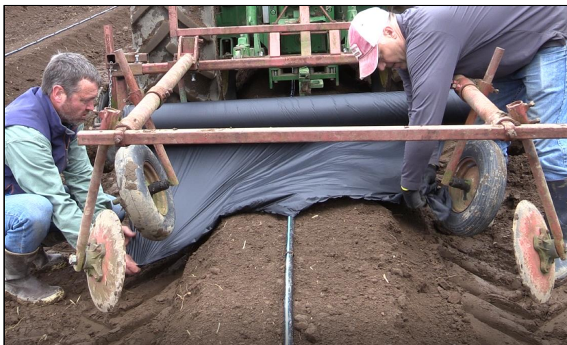
Figure 6. Load the mulch onto the layer and ensure the mulch unrolls from the bottom (photo credit to Chris Benedict).
