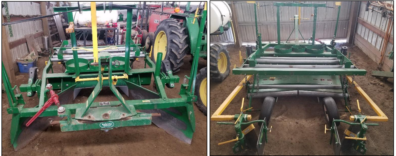
Figure 12. Bed shaper and mulch layer, front (left) and back (right) (photo credit to Lisa DeVetter).
