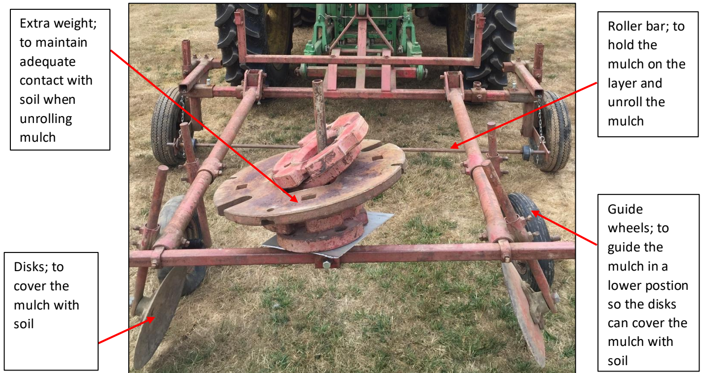
Figure 3. Customized flatbed layer used to apply plastic mulch (biodegradable or nondegradable).
